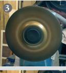
3 Leave the lathe spinning for a minute or two to allow the paints to spread out. On this platter each colour was added about three times. Other colour combinations, or just a single colour, can look very effective too.
