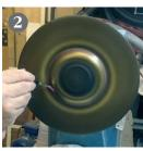
With the lathe spinning fast (1000 rpm minimum), apply the Iridescent Paints using a paint brush. Yellow and Cerise have been used here. If you don't want the colours to blend together, allow them to dry before adding another.
